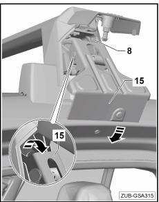
Check the exact installation position of the carrier unit – the positioning bolts of the claw fastener -15- must be positioned precisely below the mounting hole -arrow-. Move the roof bar forwards or backwards if necessary.
